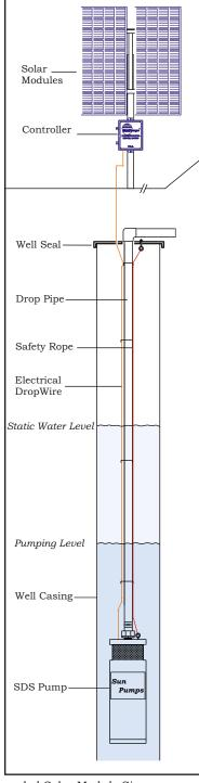
Minimum Recommended Solar Module Sizes Non shaded areas - Two 50 to 60 watt modules wired in series. Shaded areas - Two 60 to 70 watt modules wired in series. Shaded areas - Two 70 to 80 watt modules wired in series.
